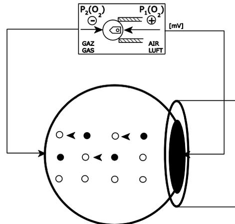
Sensor voltage depends solely on the composition of the furnace atmosphere and temperature of the furnace. The mVs measured across the sensor are a function of the carbon potential for a given temperature and CO level. The oxygen concentration of the furnace atmosphere can be
